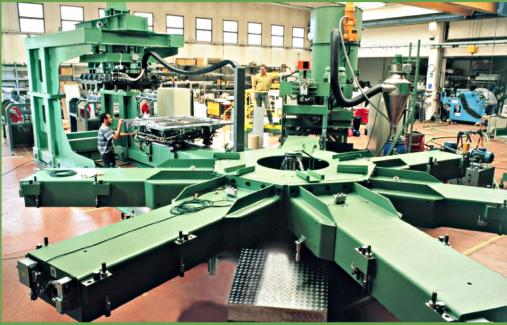
IMT extruders create the precise combination of pressure, heat and process duration required to melt the highest melting point plastics without burning or crystallizing the lowest melting point materials. The result is a highly cohesive, moldable material which is fed into specialized profile or multi-dimensional molds to create an incredible variety of products.
